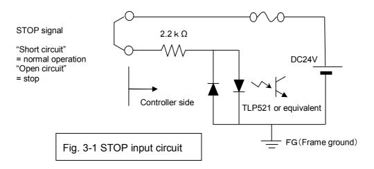
(Caution) Turn off the controller power, while connecting the stop signal input.
