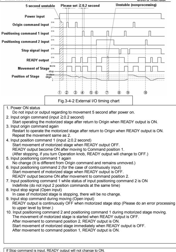
If Stop command is input, READY output will not change to ON. Even though Operation changing switch (CONT) has I/O signal, Stop switch of Panel is effective on constant basis.
