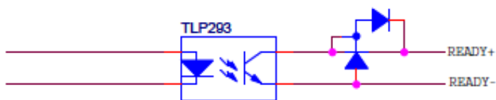
Fig4-2 Output circuits (READY)
