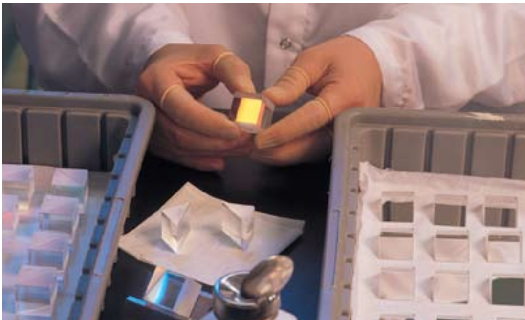
Our beamsplitter cube assembly takes place in a clean room environment to ensure high quality.
